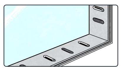
At the end of the assembly, check that the frame is level in the opening, and that the frame Is secured with a screw every 300mm at least.
