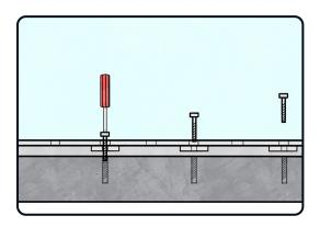
The frame is secured with supplied Keep Safe System screws or other Keep-approved screws. Note, for the frame to slide optimally, the screws must not be overtightened. This could be achieved by set screws.
