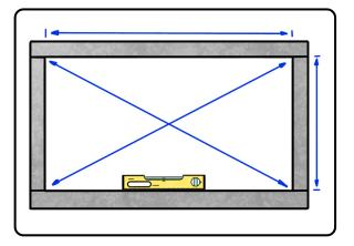
For an accepted installation the workman must have controlled that the opening is level, and all sides are within specified measurements. This is ideally done before the frame is manufactured, but not always possible.
