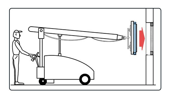
Window lifting must be done with a glass lifter, perpendicular to the opening. When lifting in, it is important that the window is parallel to the opening and that the damping is against the primary steel.
