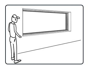
Check that the window/door opening has a correct primary steel for attachment. Also check that the access is free of debris. The workman must also check that all essential materials are available. This includes glazed frame, damping and screws.
