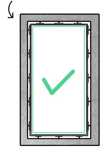
Please observe that a correctly installed frame should have an even gap to the primary steel. Therefor you should always be observant and checking the frame for any deformation, resulted by overtightening the screws.
