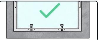
Note, for an approved installation, the window must be level and parallel in the opening. This could be achieved with the help of set screws.
