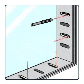
When the pane is properly aligned in the opening, the primary steel is drilled and threaded through the inner part of the oblong hole in the frame, leaving no space between the edge of the screw and edge of oblong hole. This allows the dampening element to completely compress when enough force is applied. Note, drill and thread M10 unless otherwise is specified.
